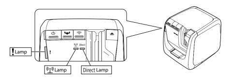
The three lamps turn off when the initialization of the network settings is complete.
