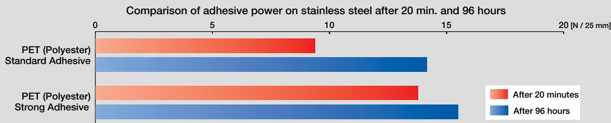
Measurements 96 hours after application (Testing method conforms to JIS Z 0237, however, the duration of application is 96H)
