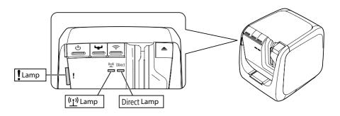
The printer power will be turned off automatically once initialization of the network settings is completed.
